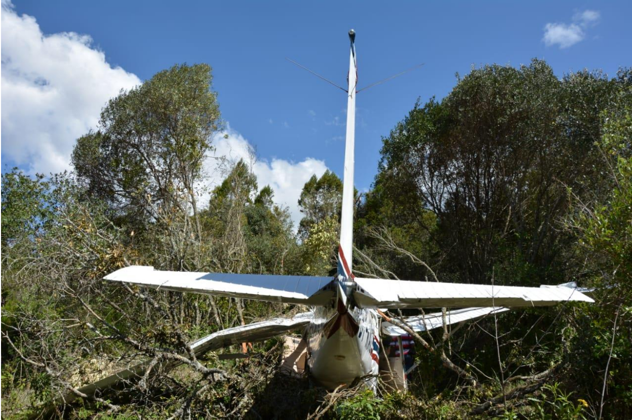
Figure 6: Photograph showing aircraft empennage section after impact
