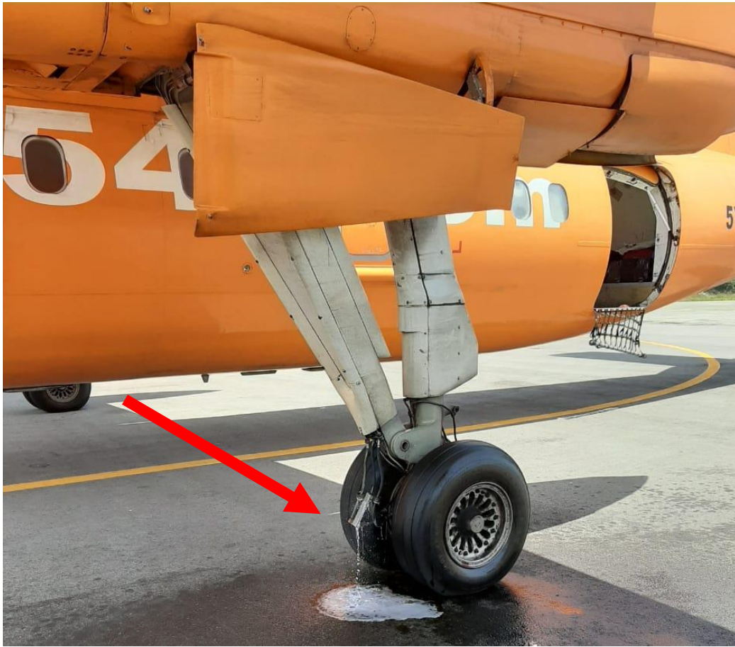
1. 5Y-CGH parked at the apron area of Malindi airport: left main landing gear brakes hydraulic leak
