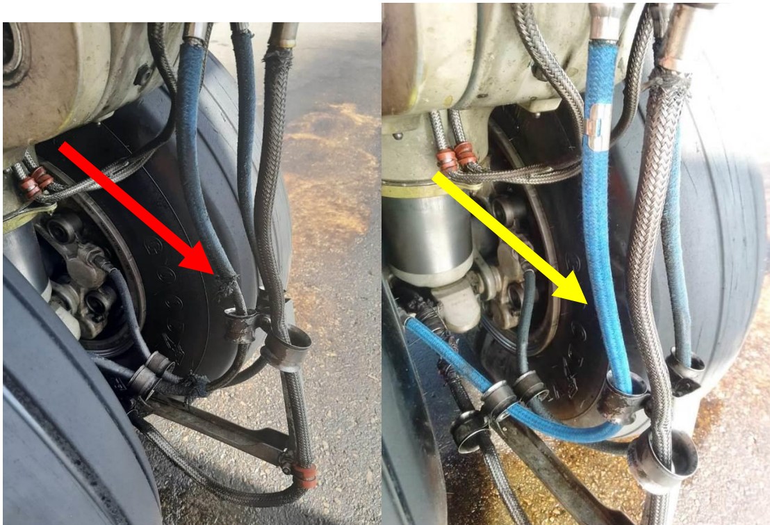
2. Photos of the affected line and its replacement respectively.
