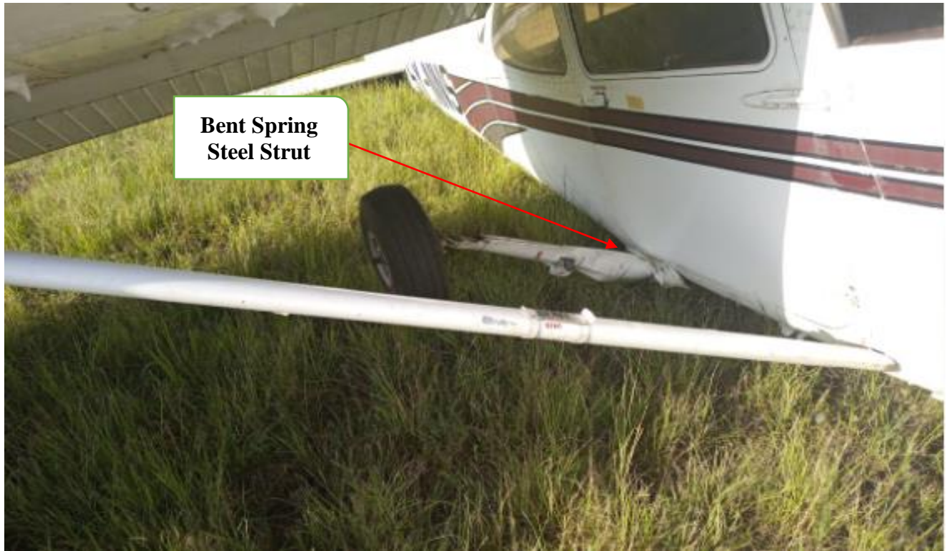
Figure 5: The section of the bent spring steel strut after the incident
