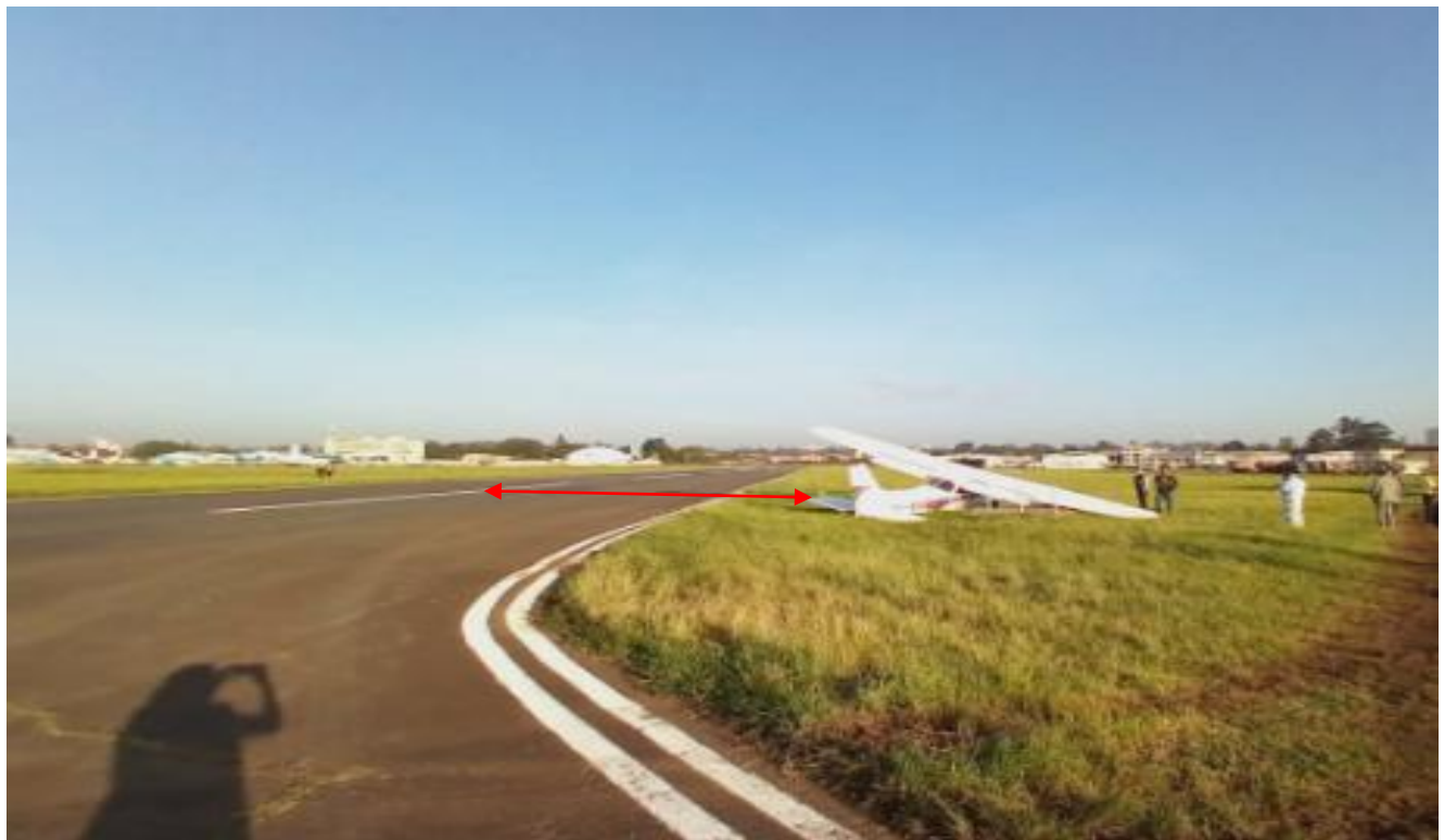
Figure 6: Final resting point from the center of the runway
