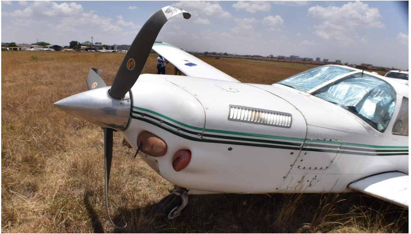
Figure 6: Damage to the propellers blades.
