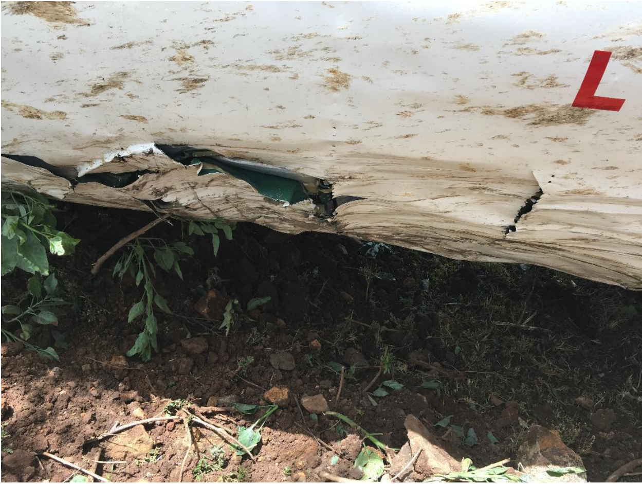
Figure 5: The ruptured skin of the Fuselage
