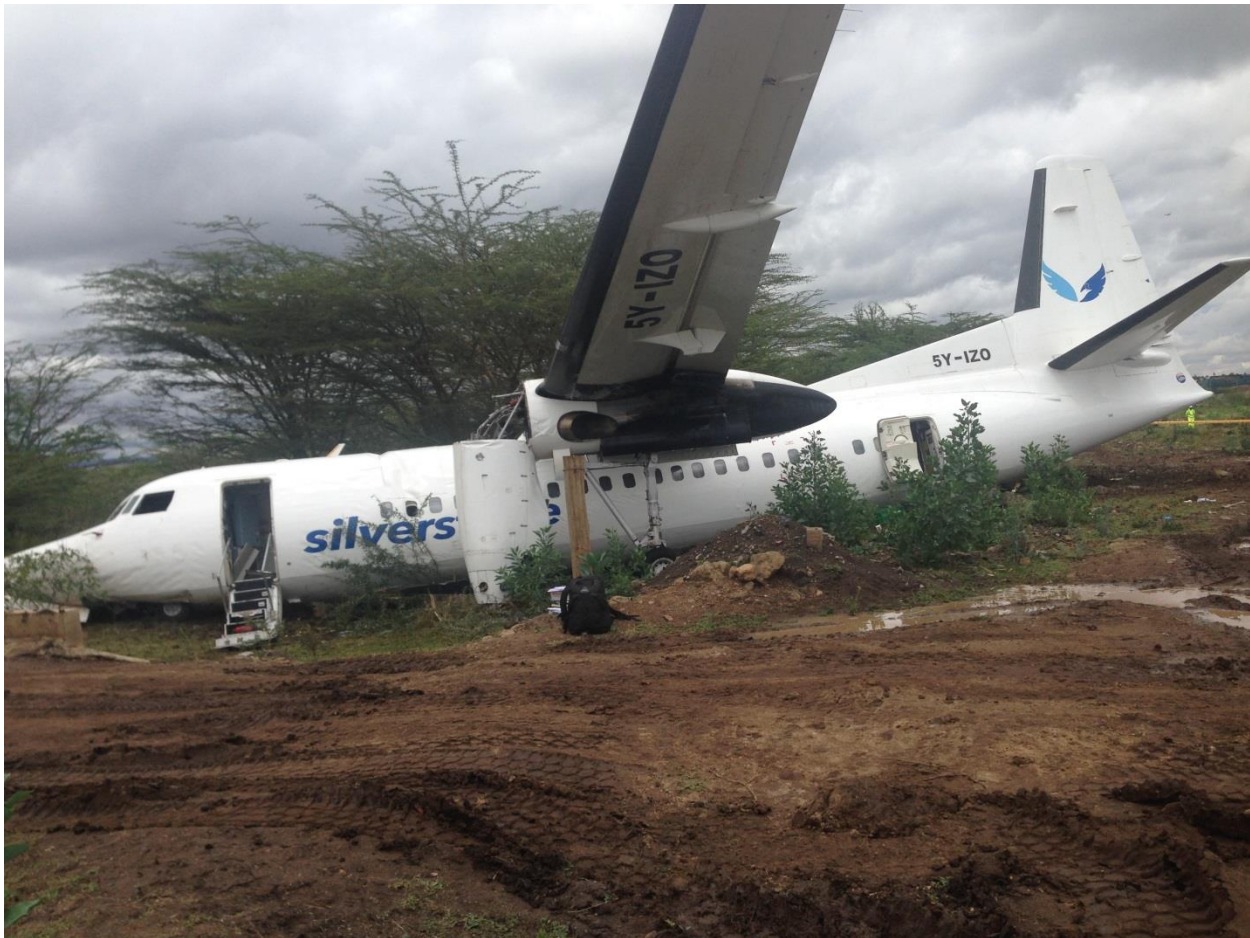
Figure 2: The detached and loosely hanging LH engine
