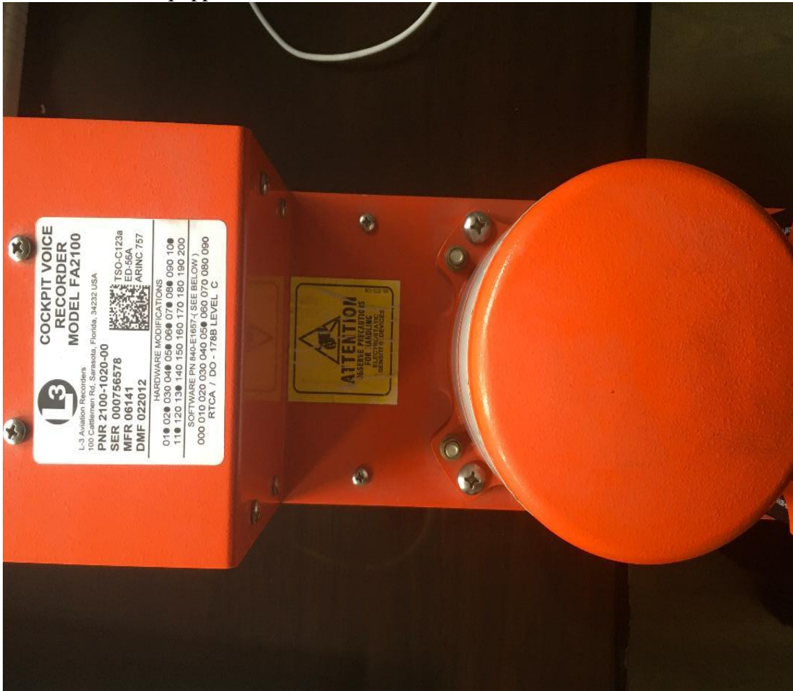
Figure 9: The Fairchild Model FA2100 CVR
