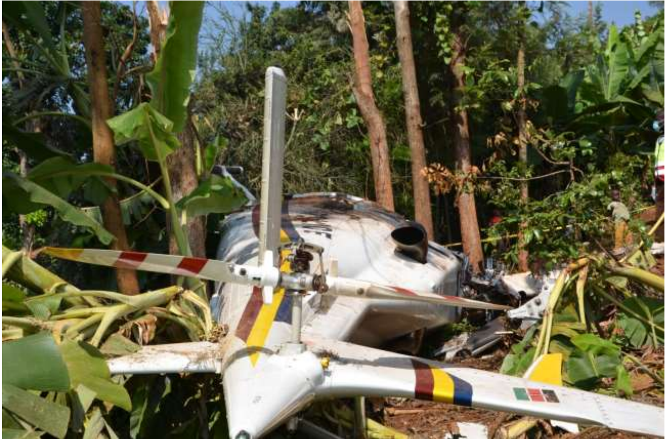
Figure 14: The helicopter tail rotor still intact
