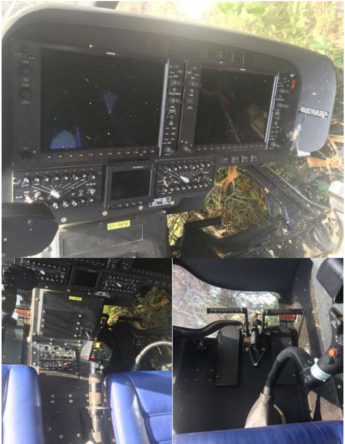
Figure 16: The cabin, cyclic, collective, throttle and the pedals
