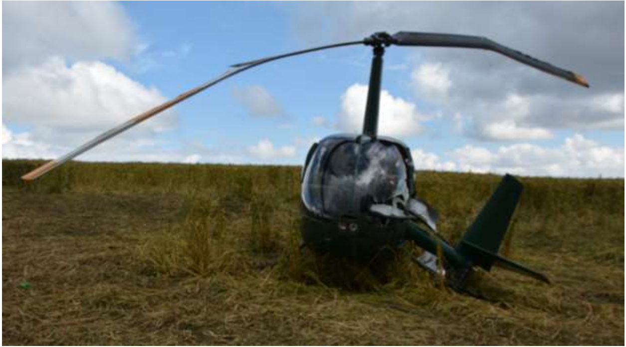
Figure 7: Helicopter Wreckage after it was tilted with the detached tail rotor on the side.
