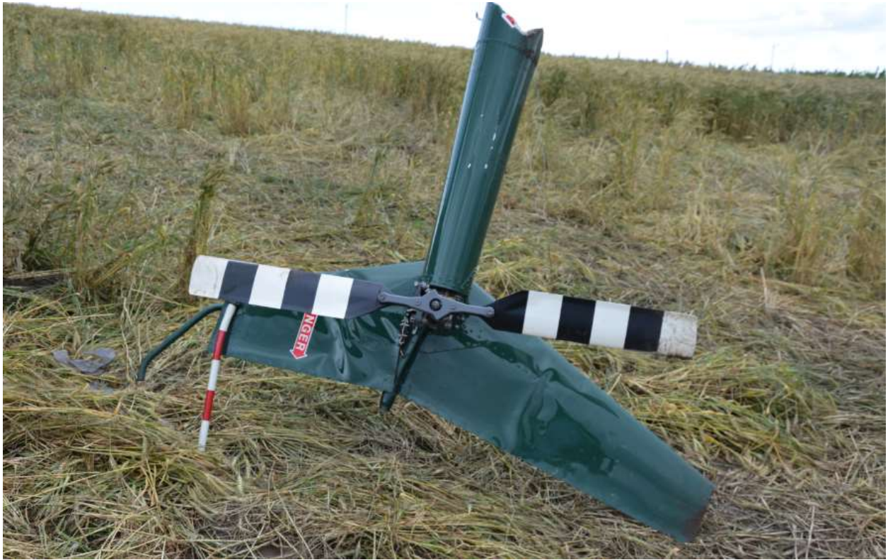
Figure 9: Damaged tail rotor assembly
