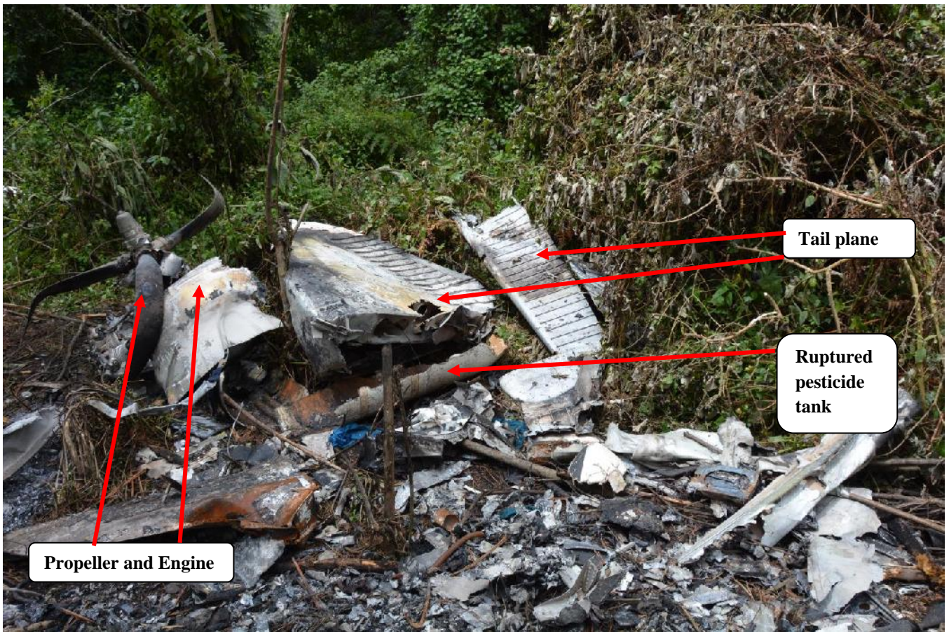
FIGURE No. 3 - Accident site (engine, propeller and tail plane)
