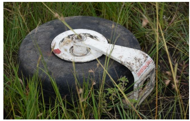
Photo 1: The C206, 5Y-CHR accident site; Photo 2: The detached nose landing gear
