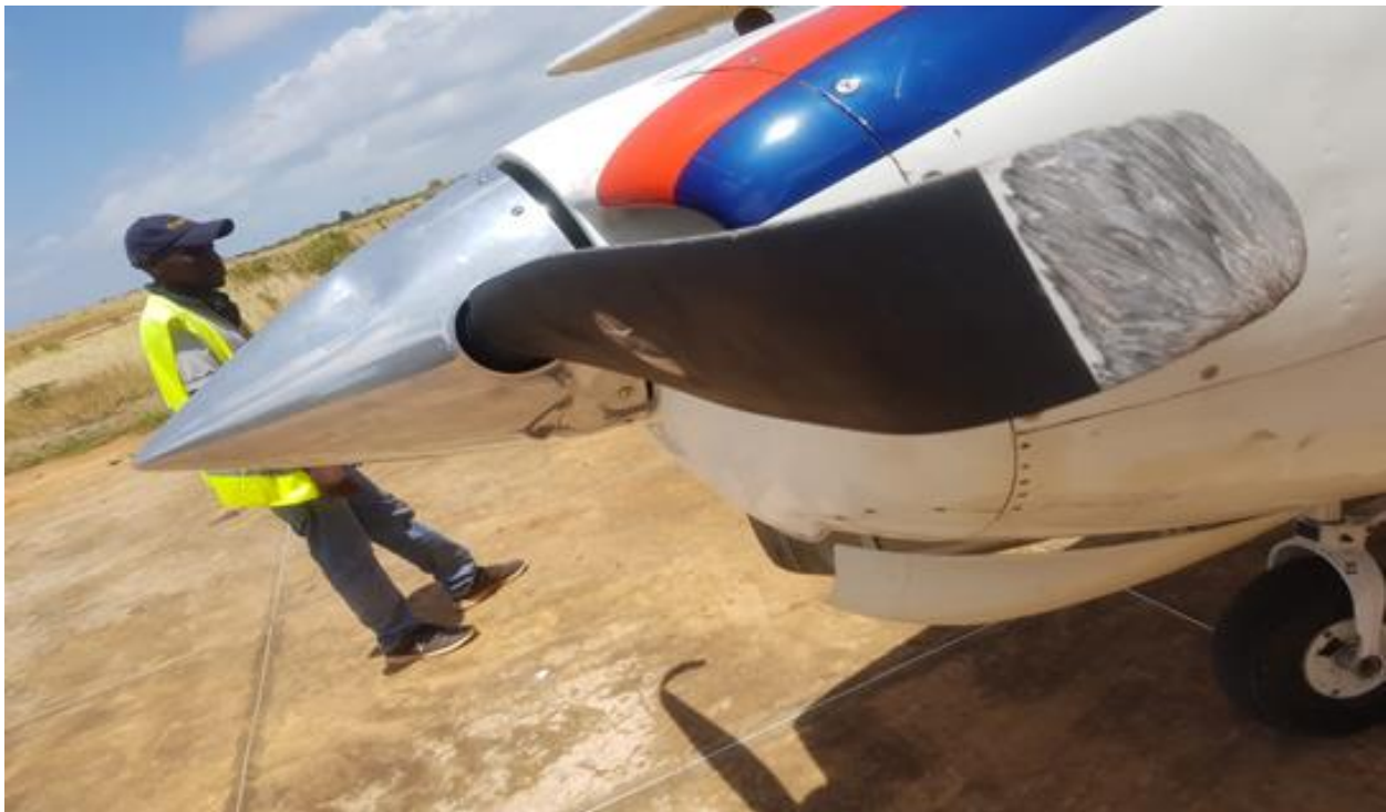
Figure 4: Damage to the propeller
