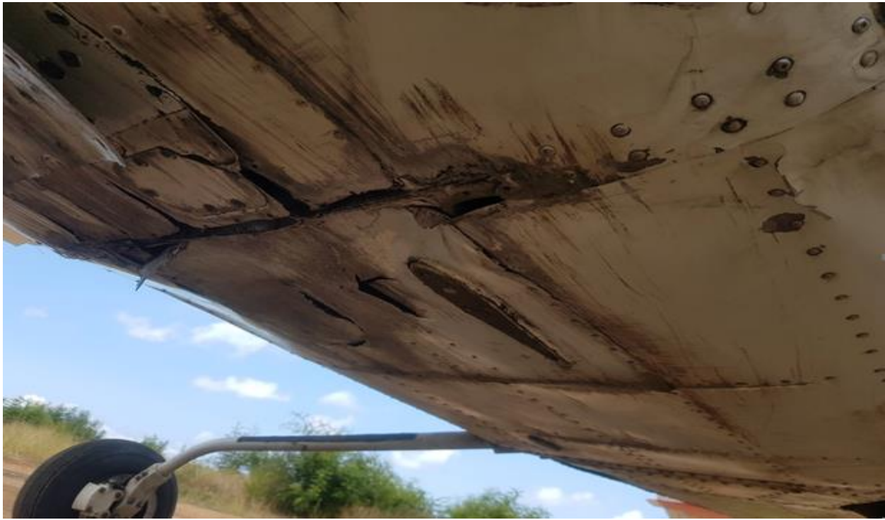
Figure 6: Damage to the outer skin on the bottom of the fuselage
