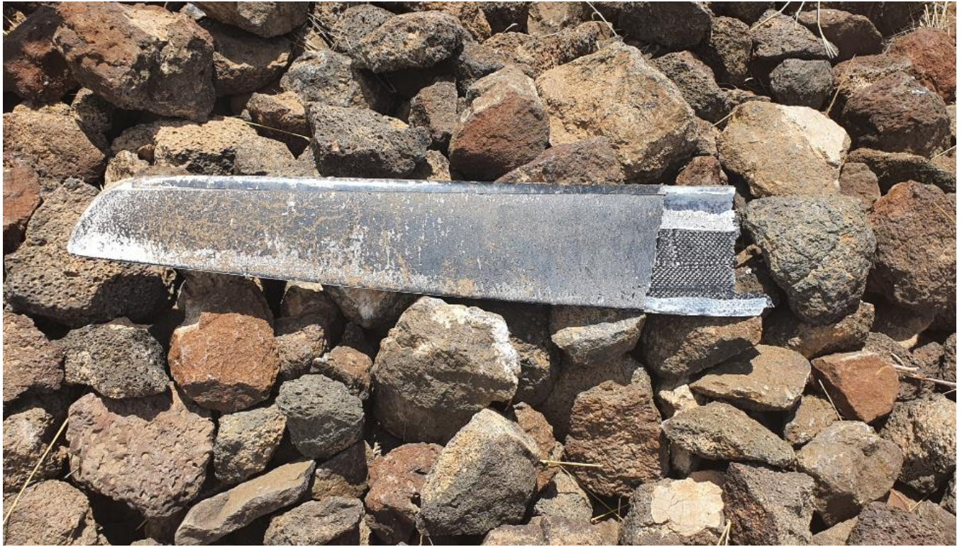
Figure 7: Broken Propeller blade
