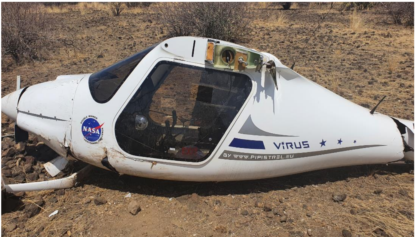
Figure 6: LH of the accident aircraft with the wing detached
