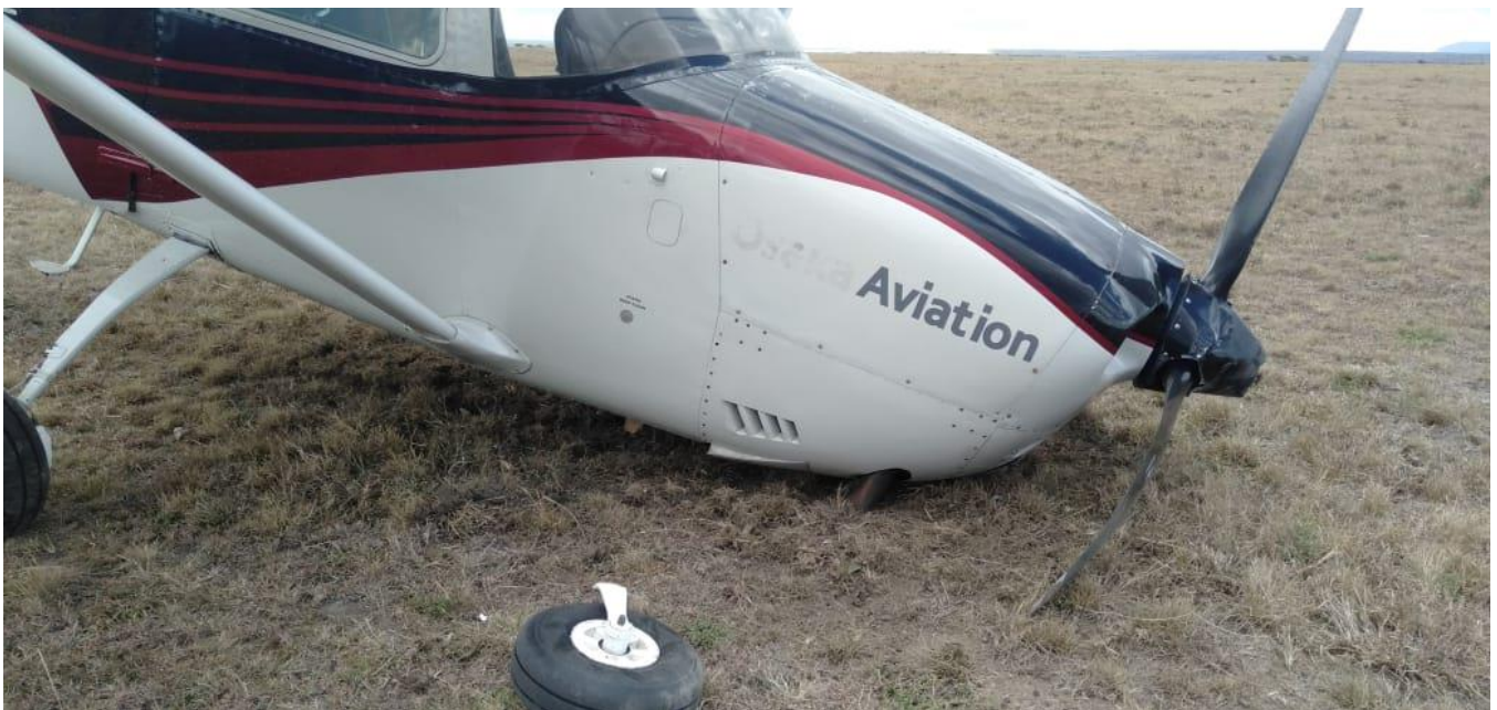
FIGURE No. 2 – A photo depicting extent of damage to the propeller and nose landing gear wheel.
