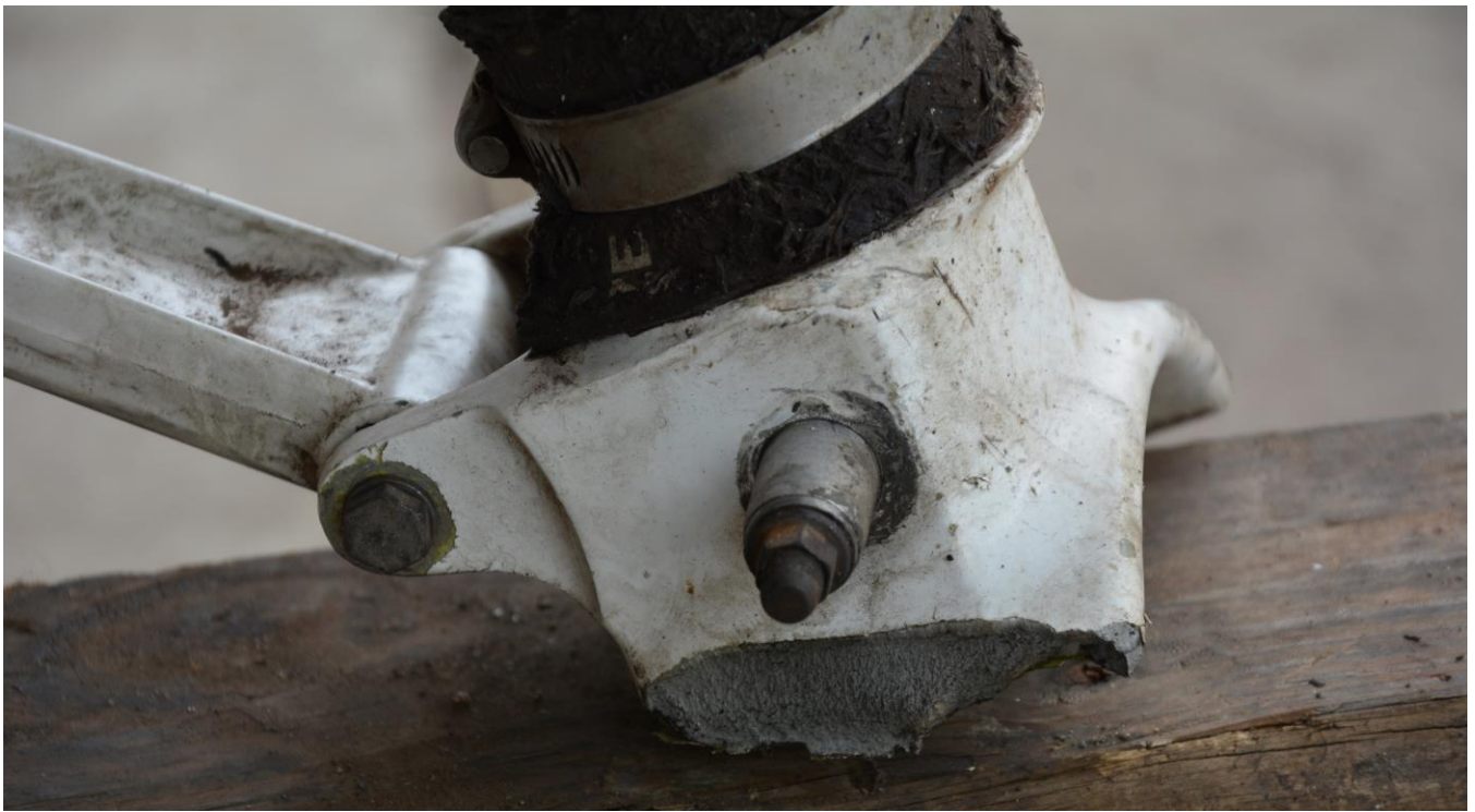
FIGURE No. 7 – Broken nose gear fork
