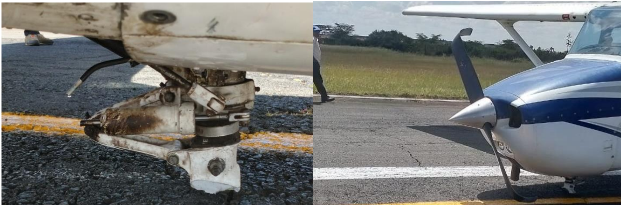
FIGURE No. 2 and 3 – Photos depicting extent of damage to the propeller and nose landing gear wheel.
