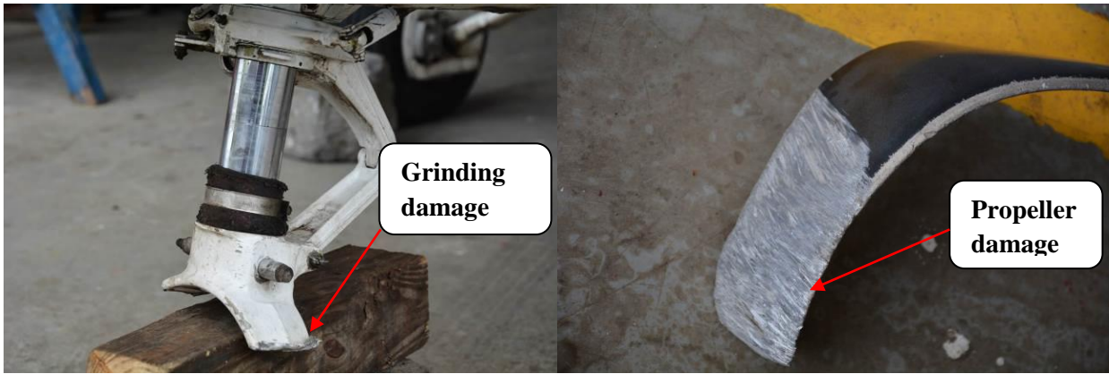
FIGURE No. 4 and 5 – Photo depicting damage of nose landing gear and propeller.
