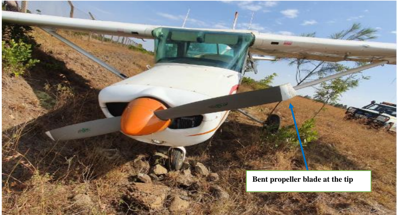
Figure 4: The front section of the aircraft after the final stop
