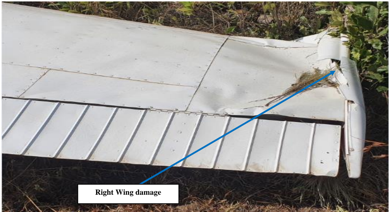
Figure 7: Right-wing outboard damage.
