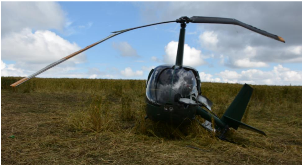
Figure 6: Helicopter Wreckage after it was tilted with the detached tail rotor on the side.
