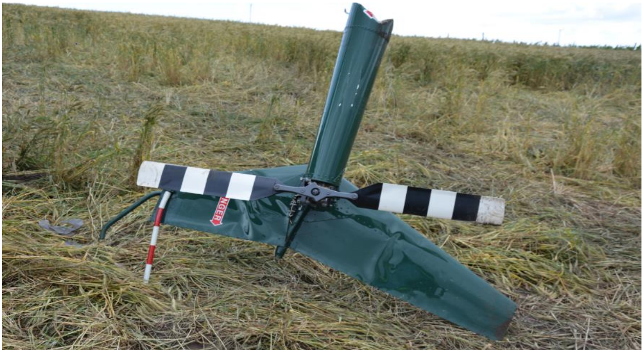
Figure 8: Damaged tail rotor assembly
