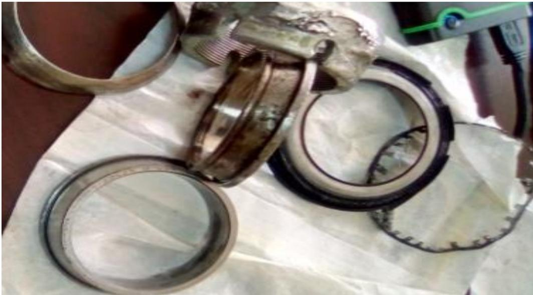
**Figure 3:** Photograph showing cone bearings on number 3 wheel assembly
