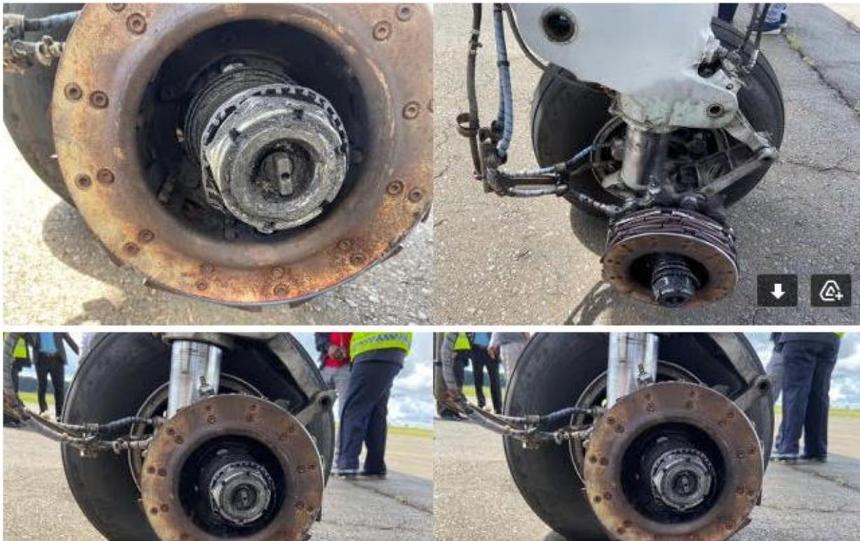
**Figure 1;** Photograph showing number 3 wheel assembly
