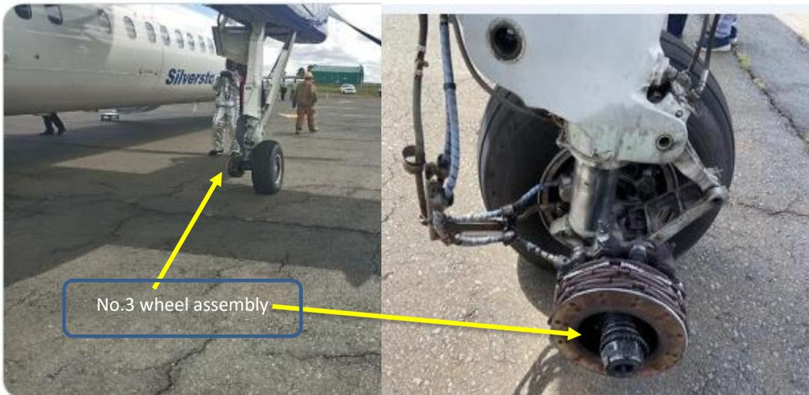
**Figure 2:** Photograph showing the aircraft and the number 3 wheel assembly
