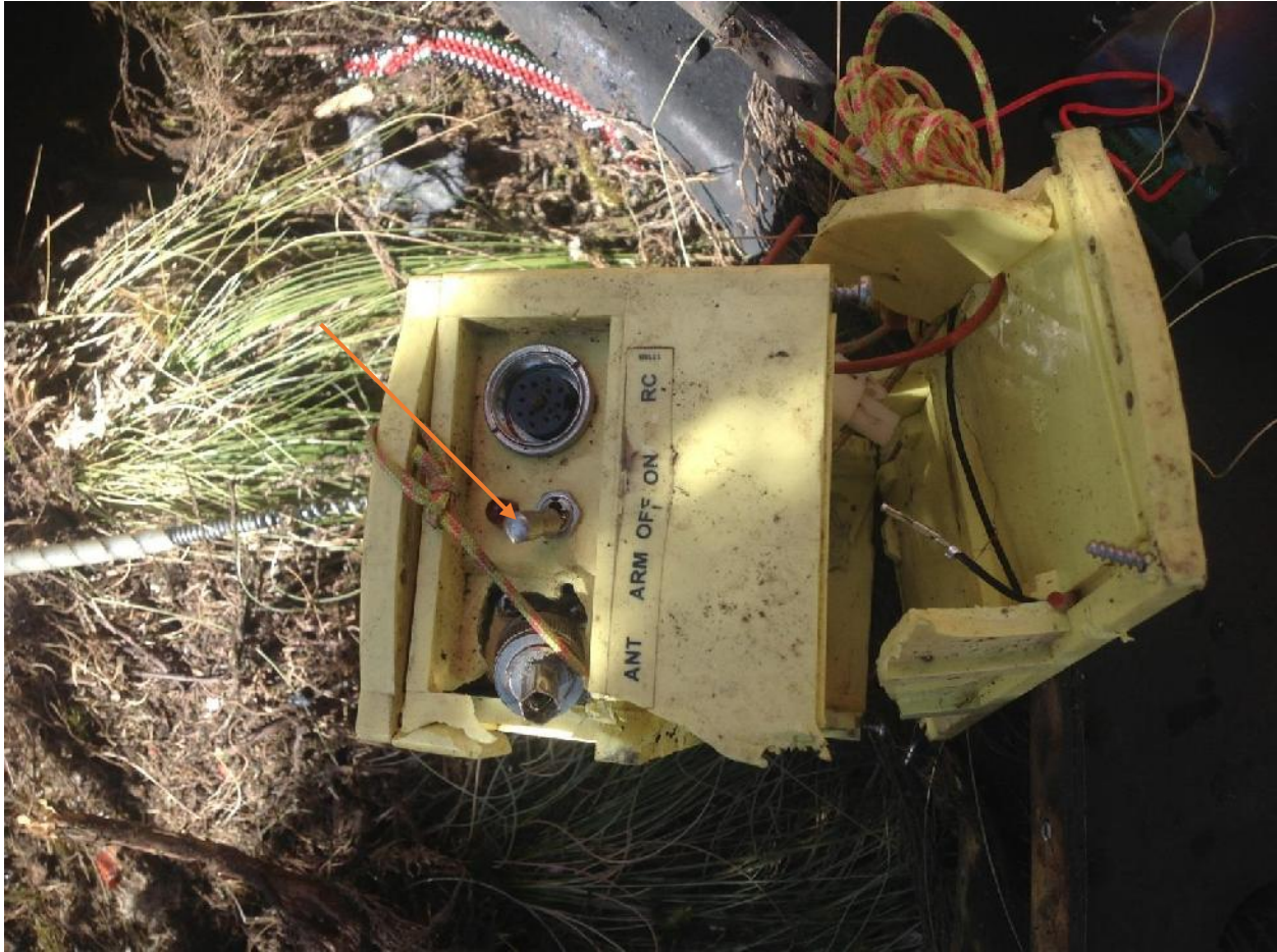
Figure 7: The damaged ELT in armed position
