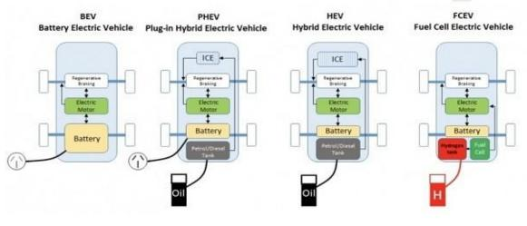
Figure 2: Types of electric vehicles Source: PT. Omazaki, 2019
