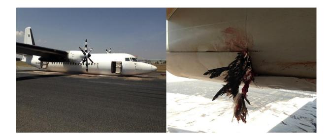
A Skyward Fokker 50, registration 5Y-SIB performing a cargo flight from Wajir to Nairobi Wilson airport was on downwind runway 07, when the crew received indication that the left main gear did not extend and lock in the down position. The crew aborted the approach and opted to extend downwind and then entered a hold, where it was confirmed the gear had not extended.
