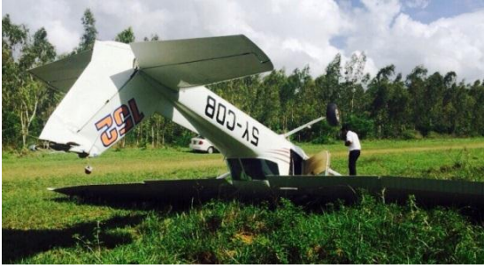
The accident aircraft lying inverted at the site
