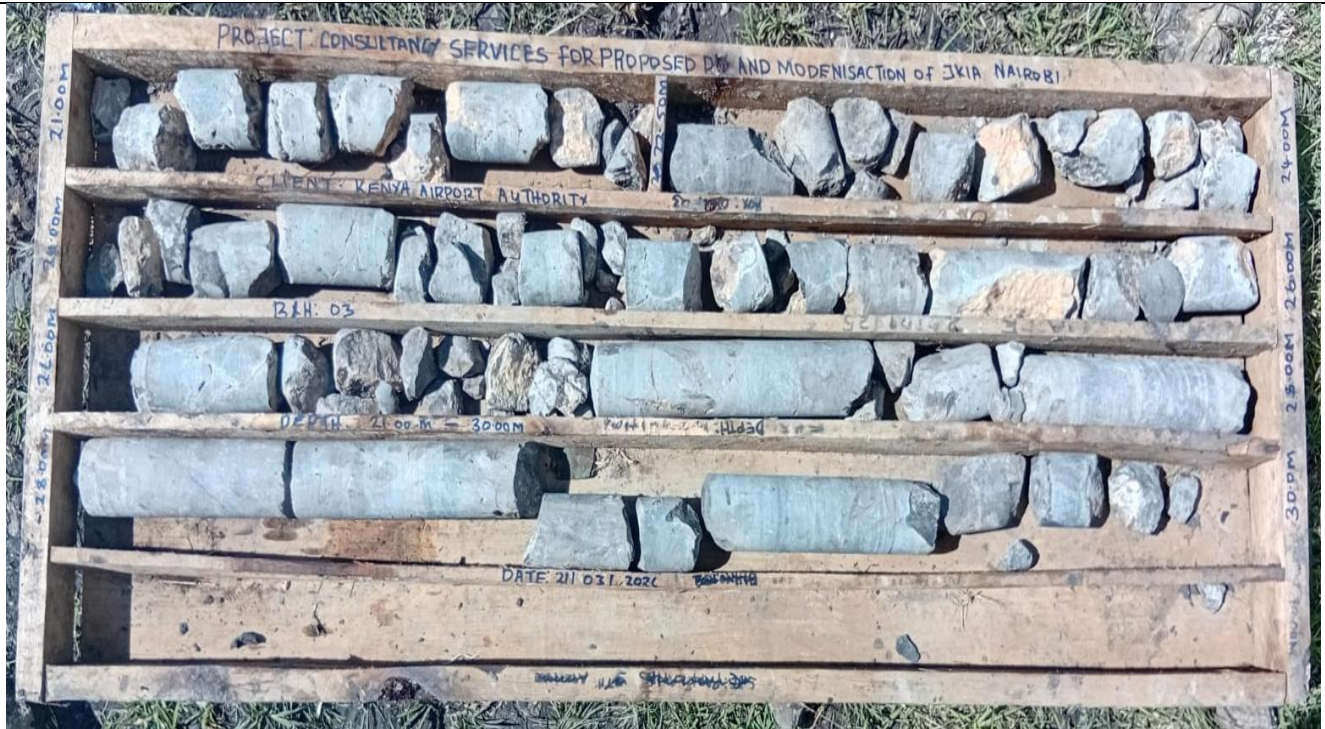
Borehole 3 depth 21.00m-30.00m
