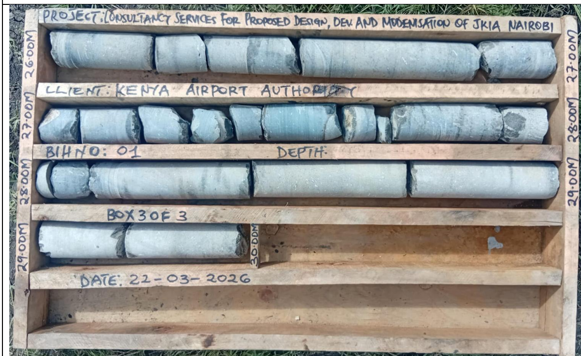
Borehole 1 depth 26.00m-30.00m
