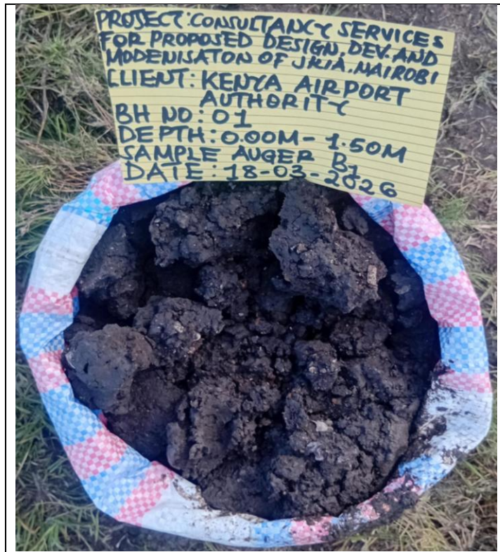
Borehole 1 depth 0.00m-1.50m
