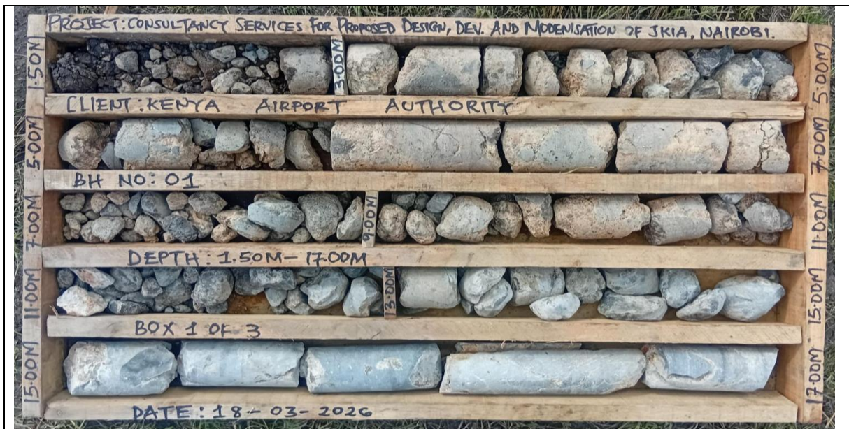
Borehole 1 depth 1.50m-17.00m
