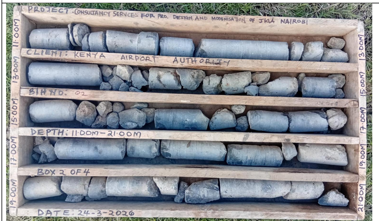
Borehole 1 depth 11.00m-21.00m
