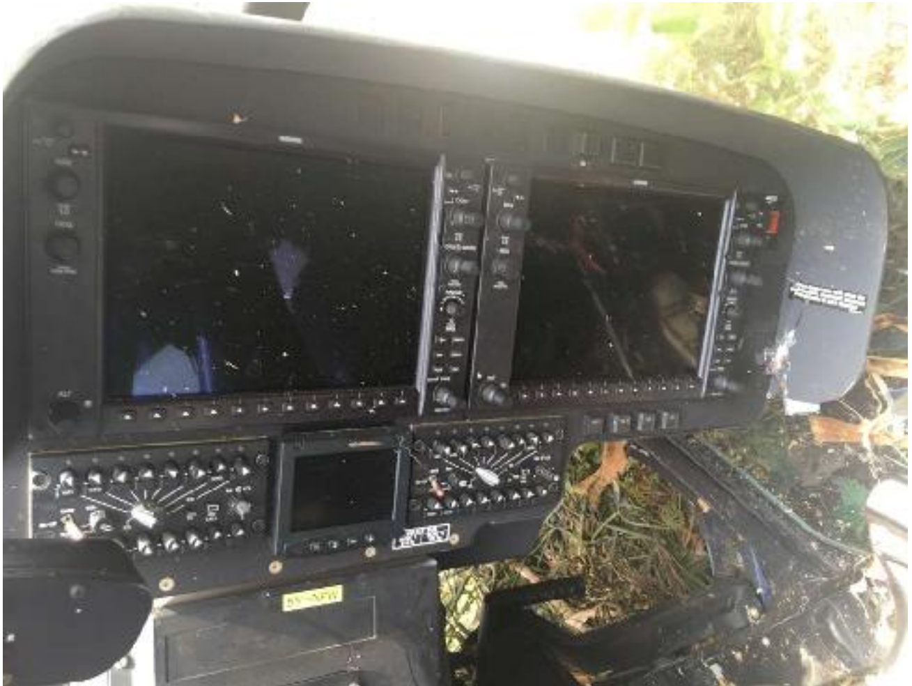
Figure 9 : ICS control panel
