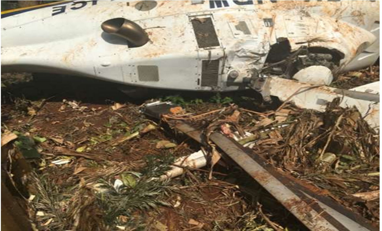
Figure 2: Main rotor blades distorted from the main rotor hub
