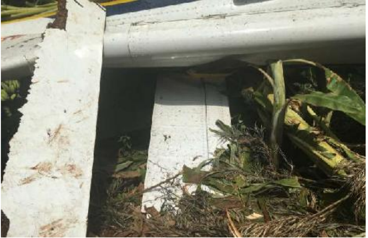
Figure 3: Damaged trailing edge of one of the main rotor blades
