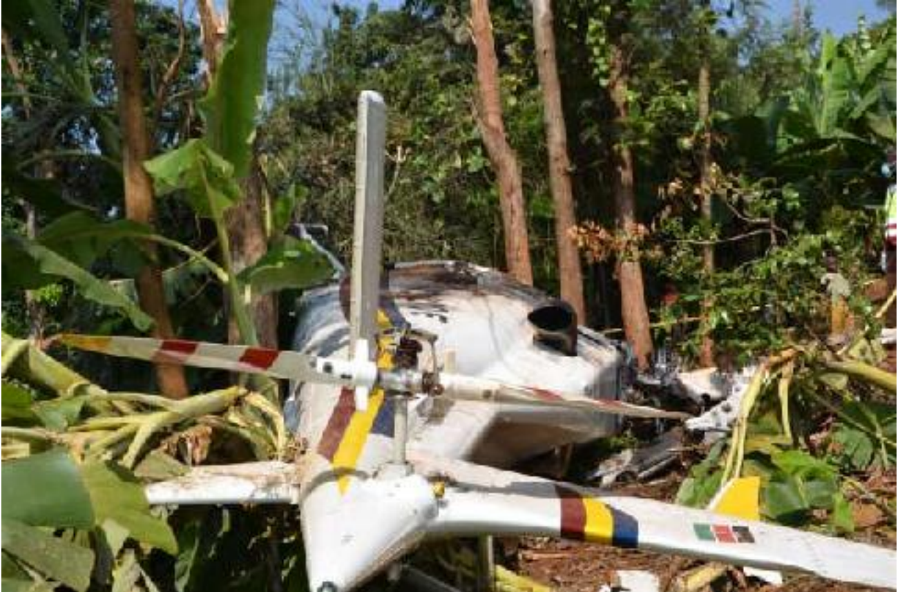
Figure 16: The helicopter tail rotor still intact
