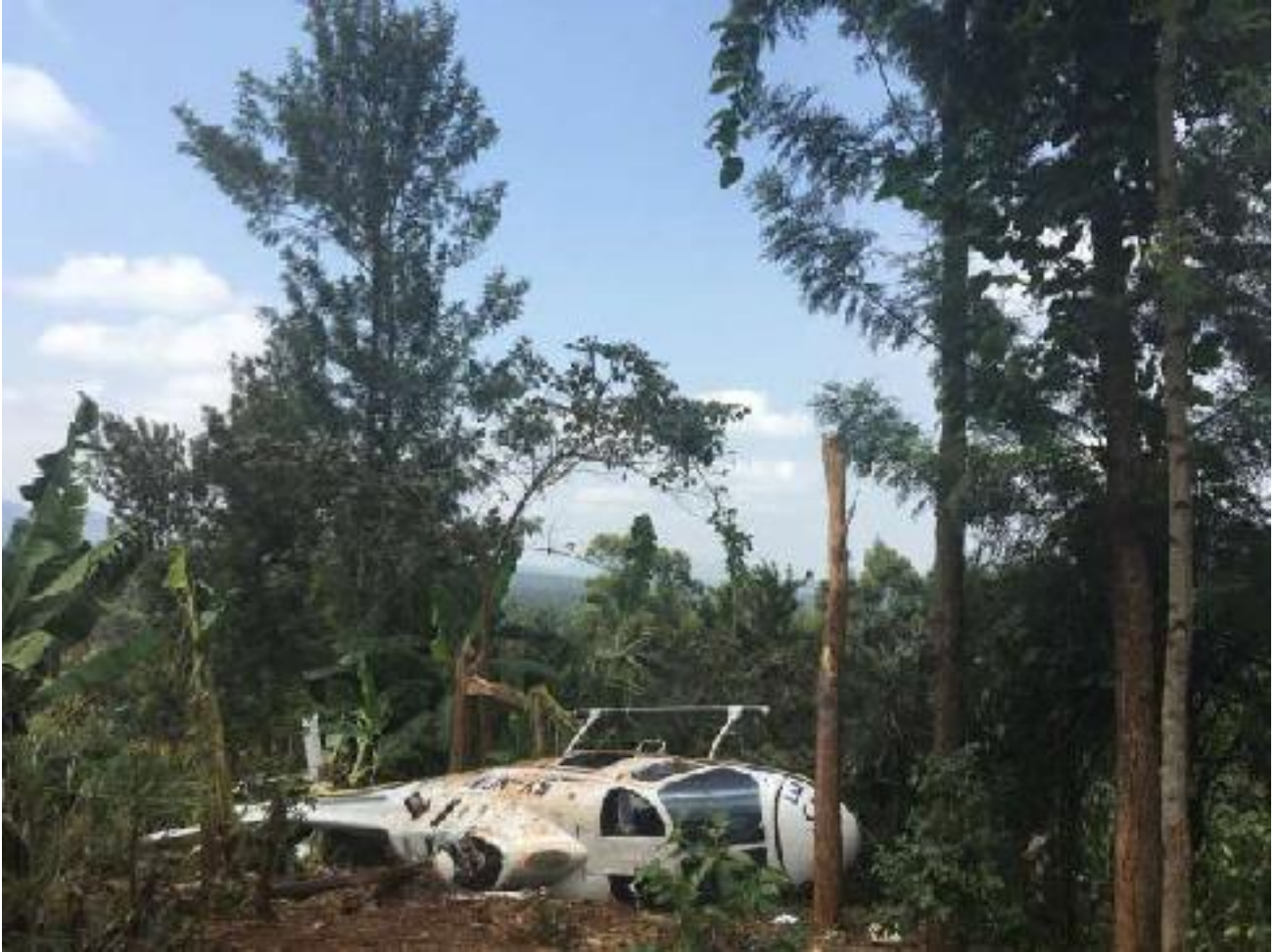
Figure 14: The wreckage and the trees that were involved in the occurrence
