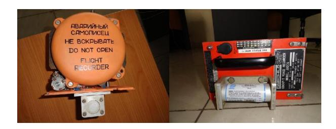
Fig 1.11.1: Flight data recorder & cockpit voice recorder recovered from the 5Y-UVP
